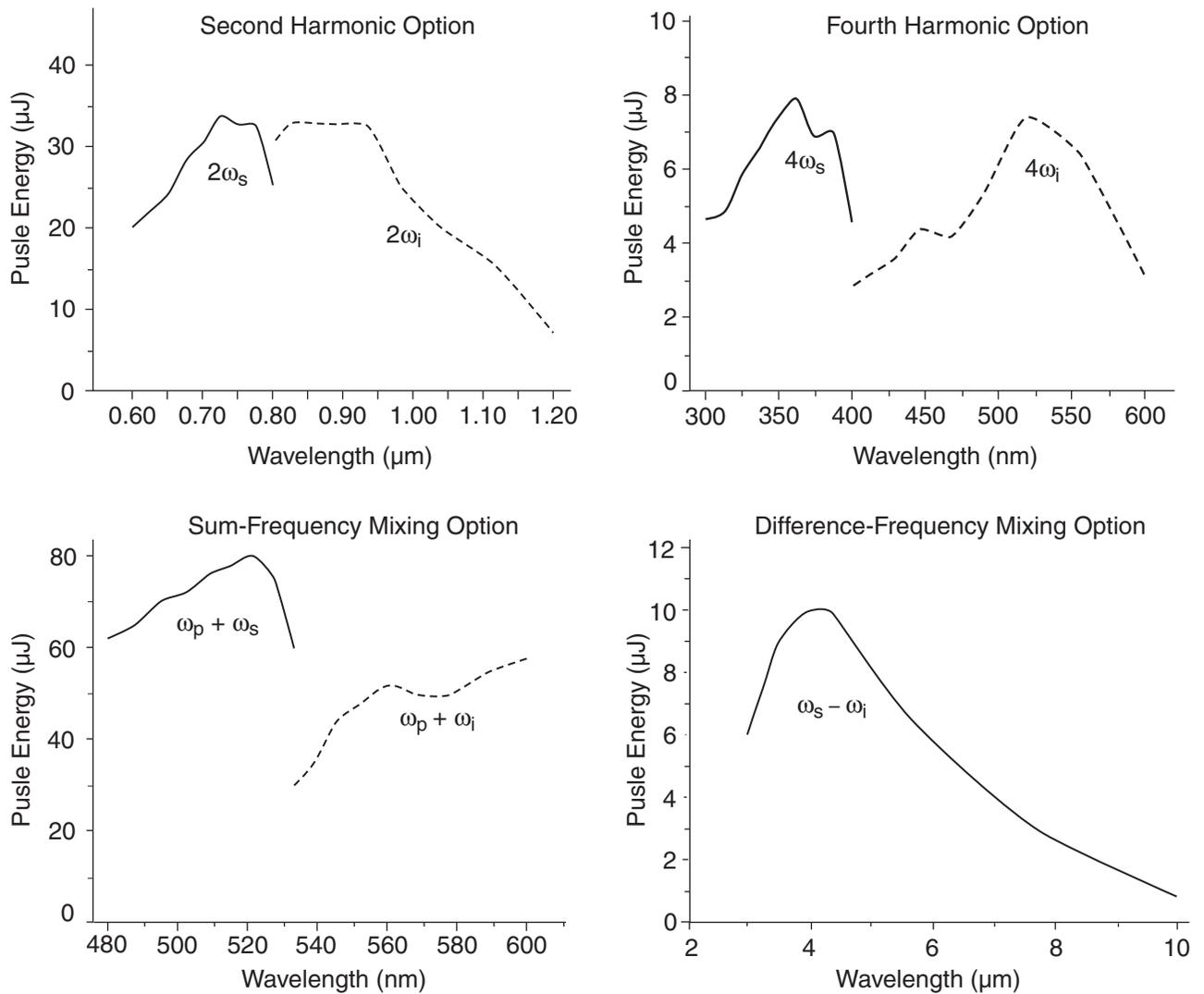
**Figure 3-7: Typical Output Tuning Curves for Wavelength Extensions for an OPA-800CF-1.**
