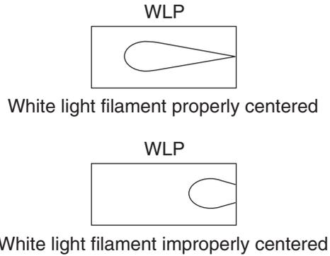
**Figure 5-3: White light filament as seen in the white light plate.**
