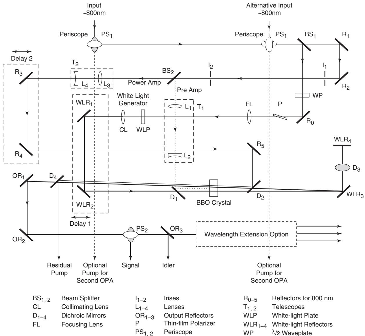
Figure 4-1: Double-Pass, Single BBO Crystal OPA-800CF
