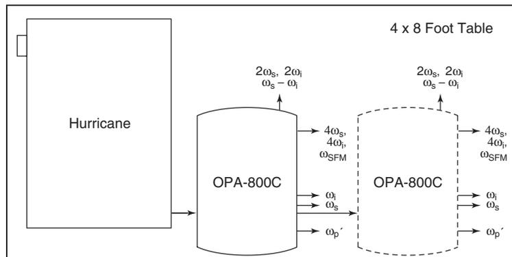
(b) A Typical Hurricane and OPA-800C System Layout (with optional second OPA)
