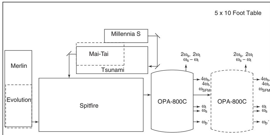
(a) A Typical Spitfire and OPA-800C System Layout (with optional second OPA)
