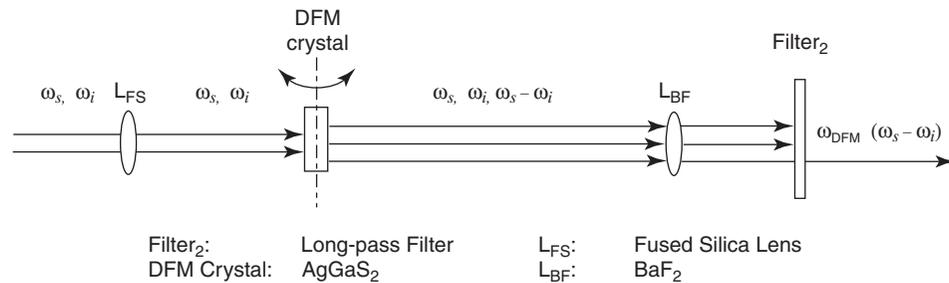
**Figure 7-9: Schematic layout of the DFM option.**
