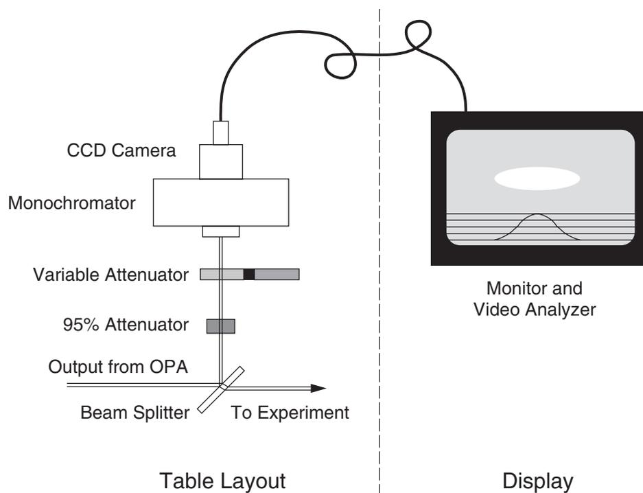
**Figure 6-2: A Typical Monochromator/CCD Camera Setup**
