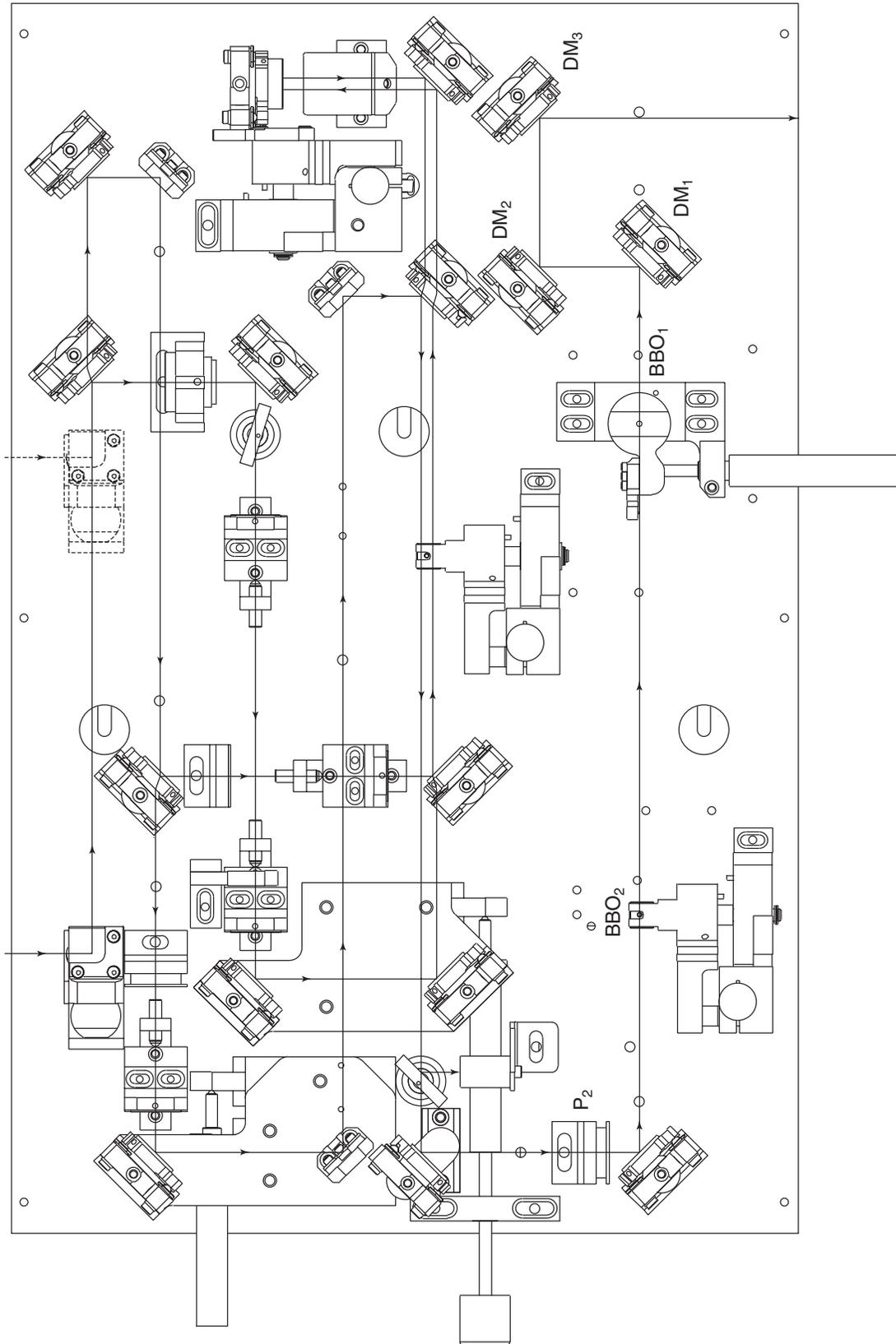
Figure 7-6: Mechanical Layout of the *OPA-800CF* Arranged for FHG of the Signal
