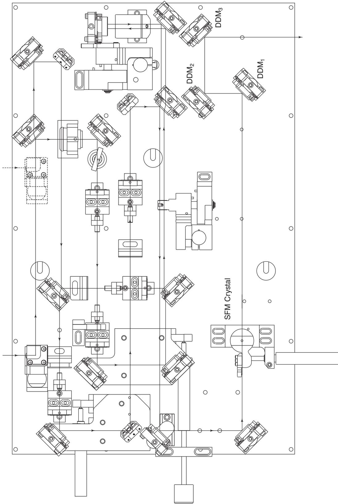
Figure 7-8: Mechanical Layout of the *OPA-800CF* Arranged for SFM
