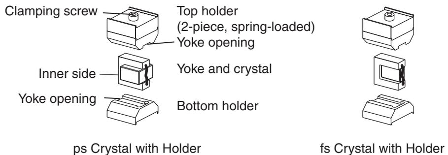
Figure 4-5: The ps and fs crystals with holders.
