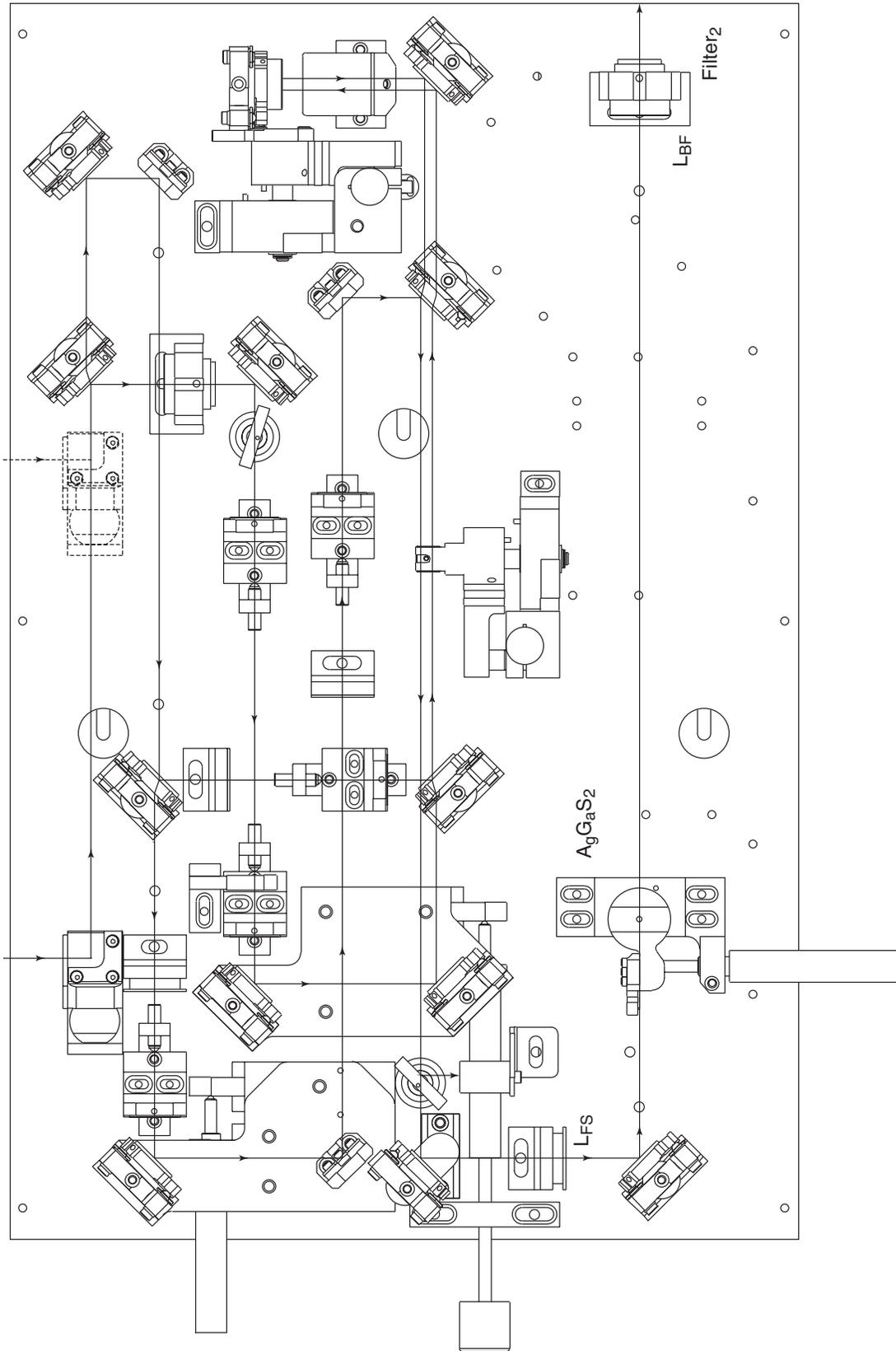
Figure 7-10: Mechanical Layout of the *OPA-800CF* Arranged for DFM
