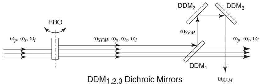
**Figure 7-7: Schematic layout of the SFM of the signal/idler with the residual pump.**
