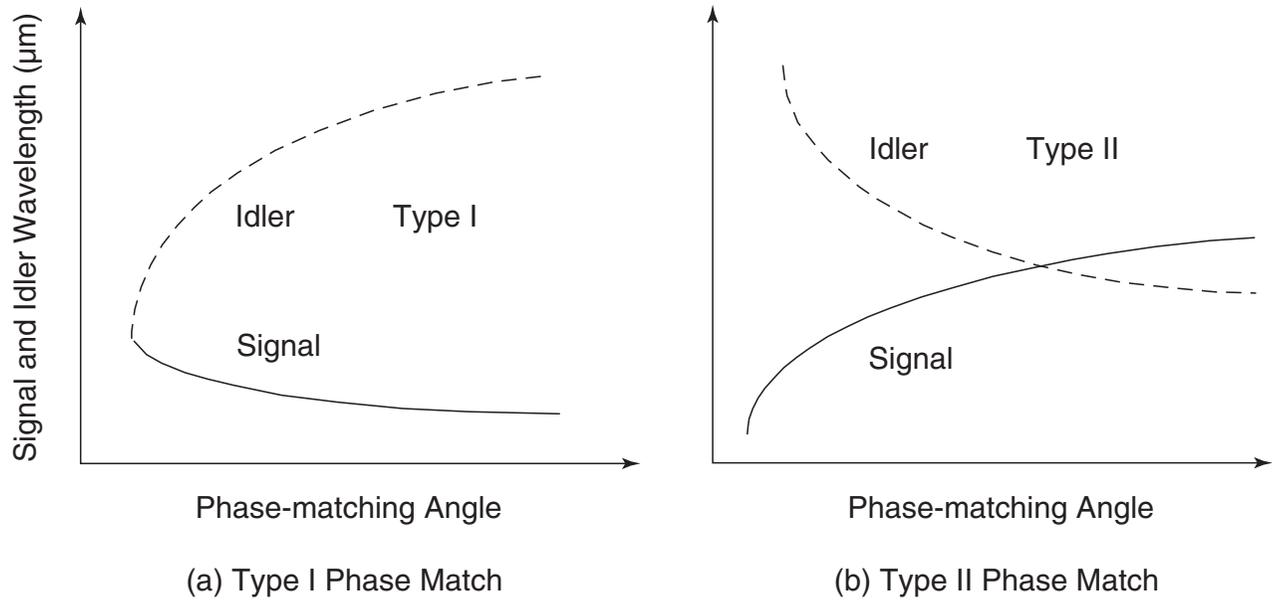
**Figure 3-4: Wavelength vs. Phase-Matching Angle of Type I and Type II Crystals**
