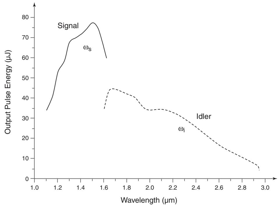
Figure 3-6: Typical Output Tuning Curves of an OPA-800CP-1.
