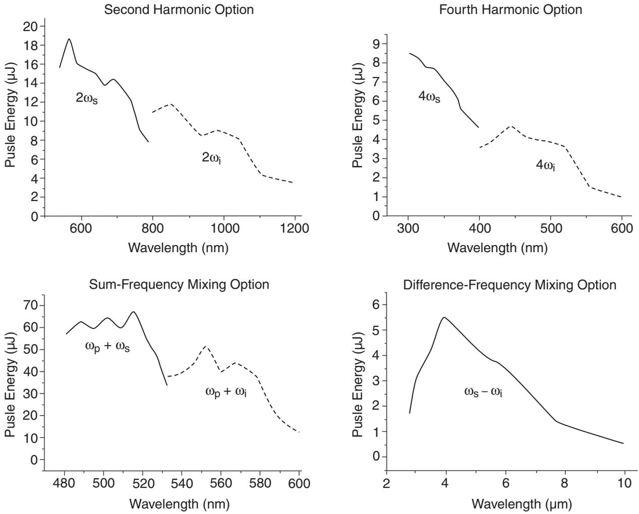
Figure 3-8: Typical Output Tuning Curves for Wavelength Extensions for an OPA-800CP-1.
