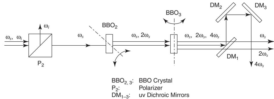
**Figure 7-5: Schematic layout of the FHG of the signal.**
