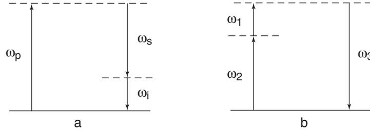
**Figure 3-1: Optical frequency three-wave interaction process**
