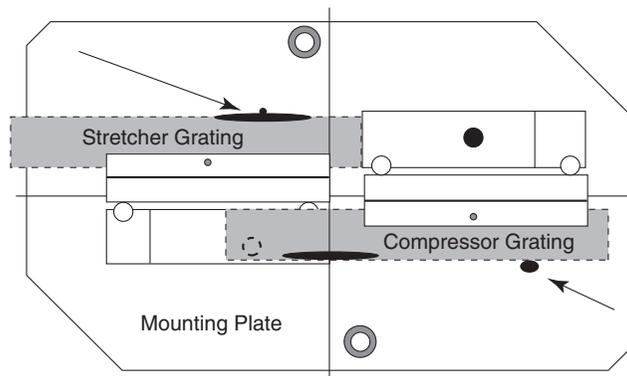
**Figure A-2: Standard Symmetrical Grating Configuration**
