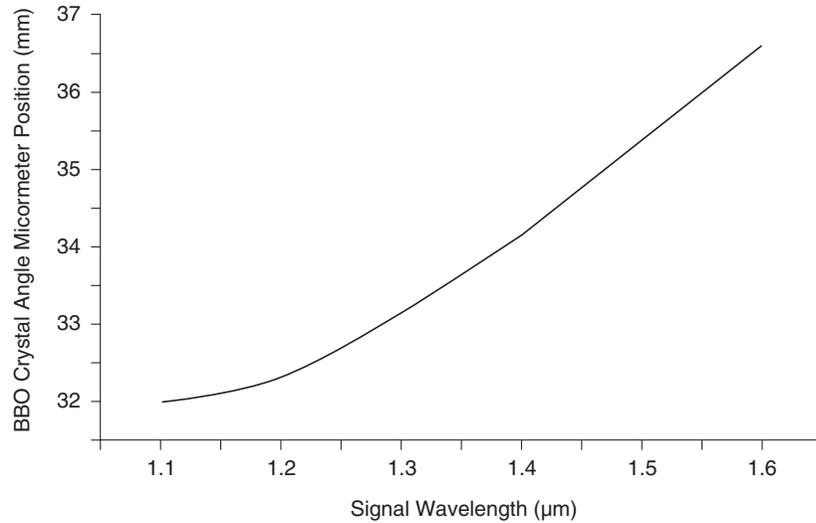
**Figure 6-3: Typical Signal Wavelength vs. BBO Crystal Angle Position**
