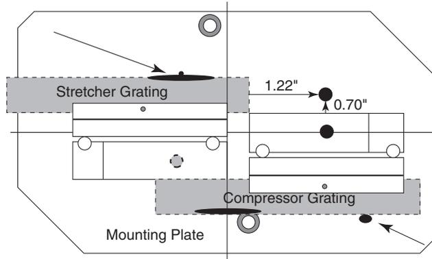
**Figure A-3: Grating Configuration Modified for ps-masked *Spitfire*.**
