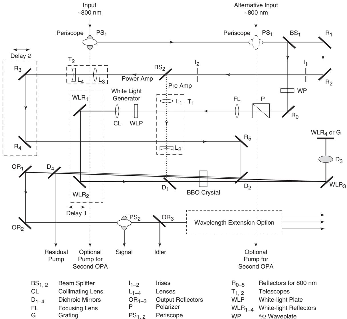
Figure 1-2: The *OPA-800C* Beam Path
