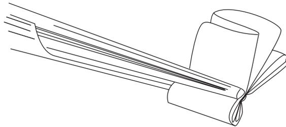
**Figure 8-1: Lens Tissue Folded for Cleaning**
