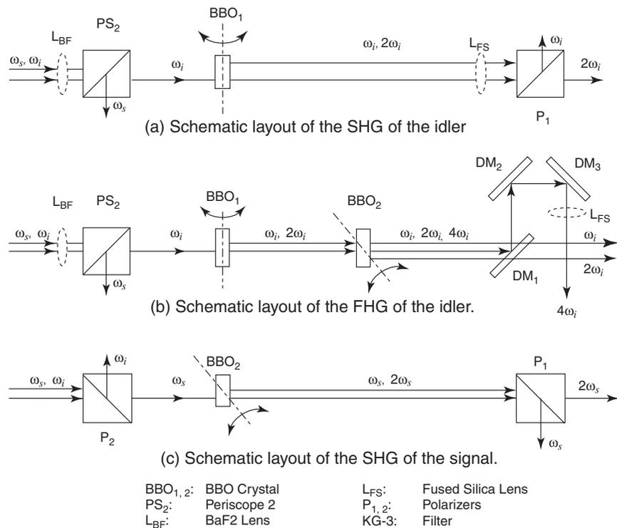
**Figure 7-4: Configuration for SHG (a) and FHG (b) of the idler and SHG of the signal (c).**
