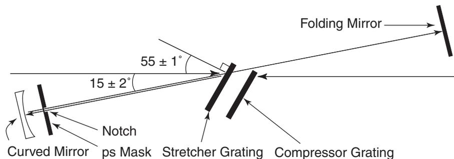
**Figure A-1: Schematic of a Stretcher with ps Mask.**
