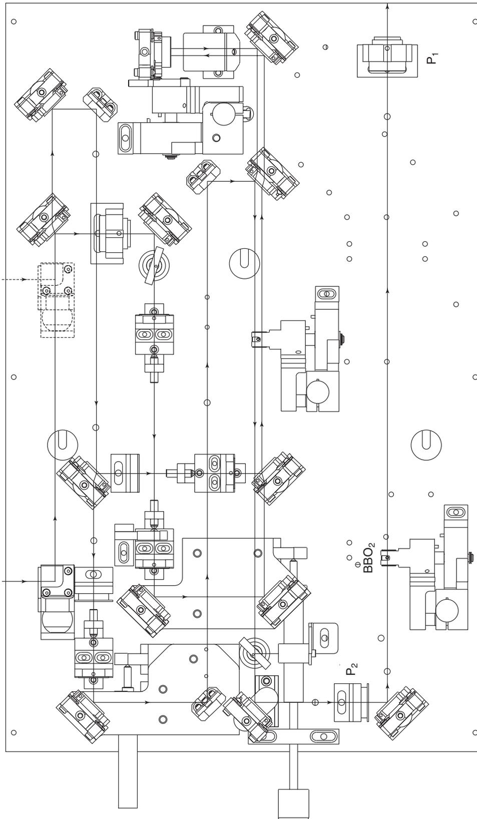
Figure 7-3: Mechanical Layout of the *OPA-800CF* Arranged for SHG of the Signal
