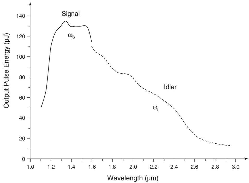
Figure 3-5: Typical Output Tuning Curves of an OPA-800CF-1.
