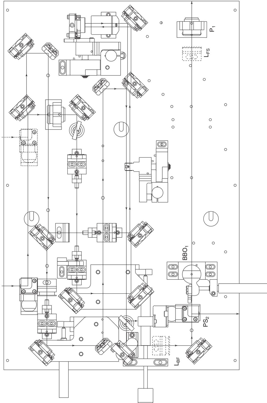
Figure 7-1: Mechanical Layout of the *OPA-800CF* Arranged for SHG of the Idler
