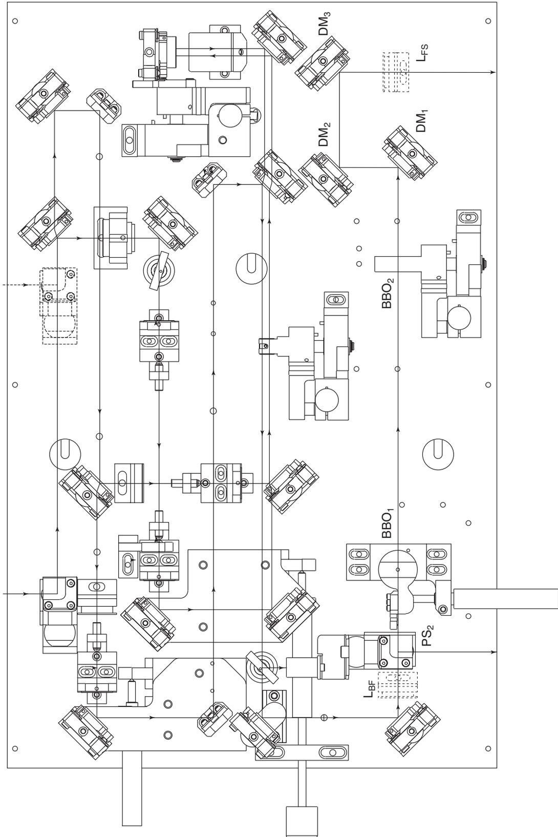
Figure 7-2: Mechanical Layout of the *OPA-800CF* Arranged for FHG of the Idler
