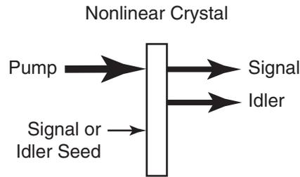
**Figure 3-2: Optical Parametric Amplification**
